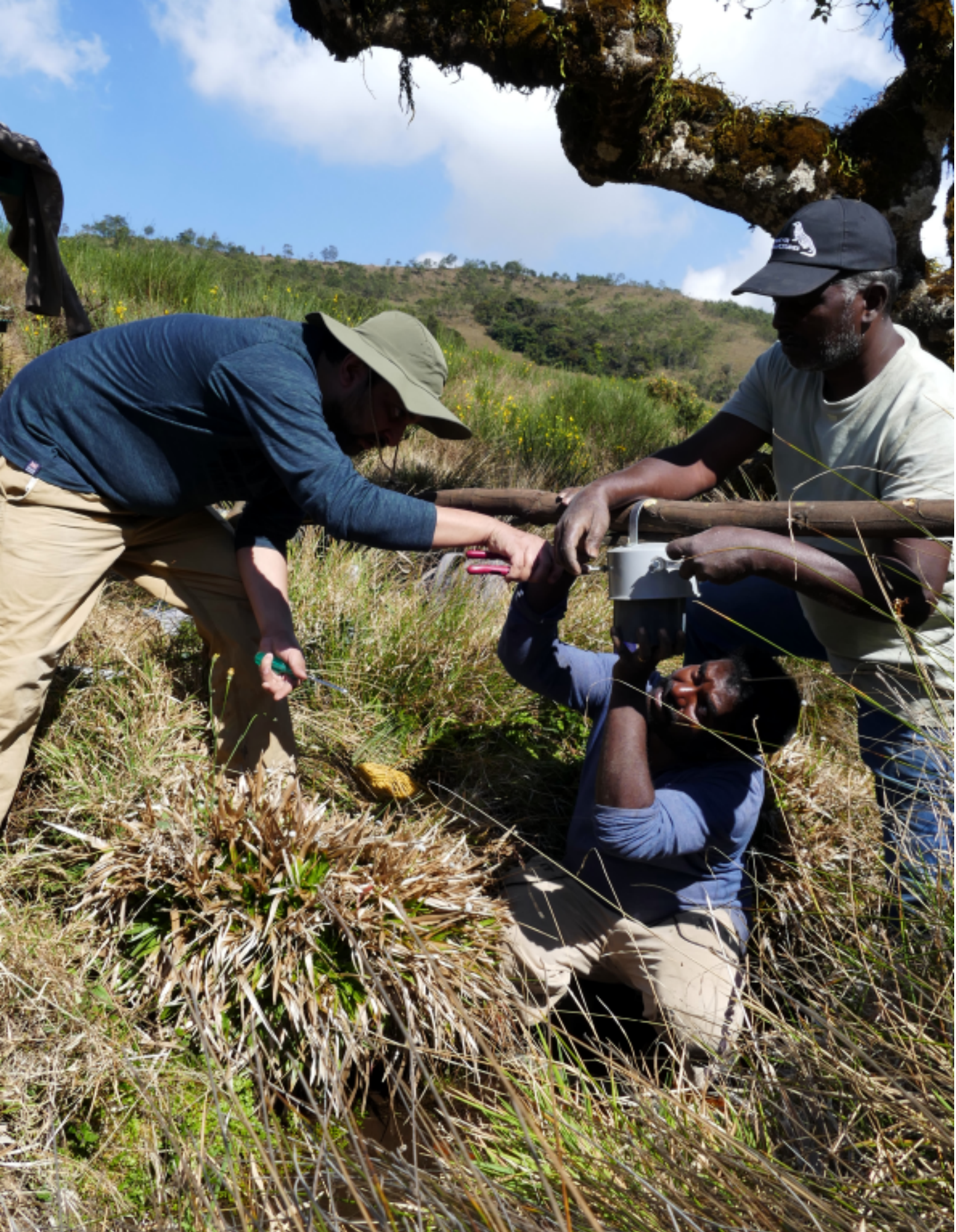
Using acoustic-based water level recorders, we monitored stream levels across a gradient of wattle invasion.
